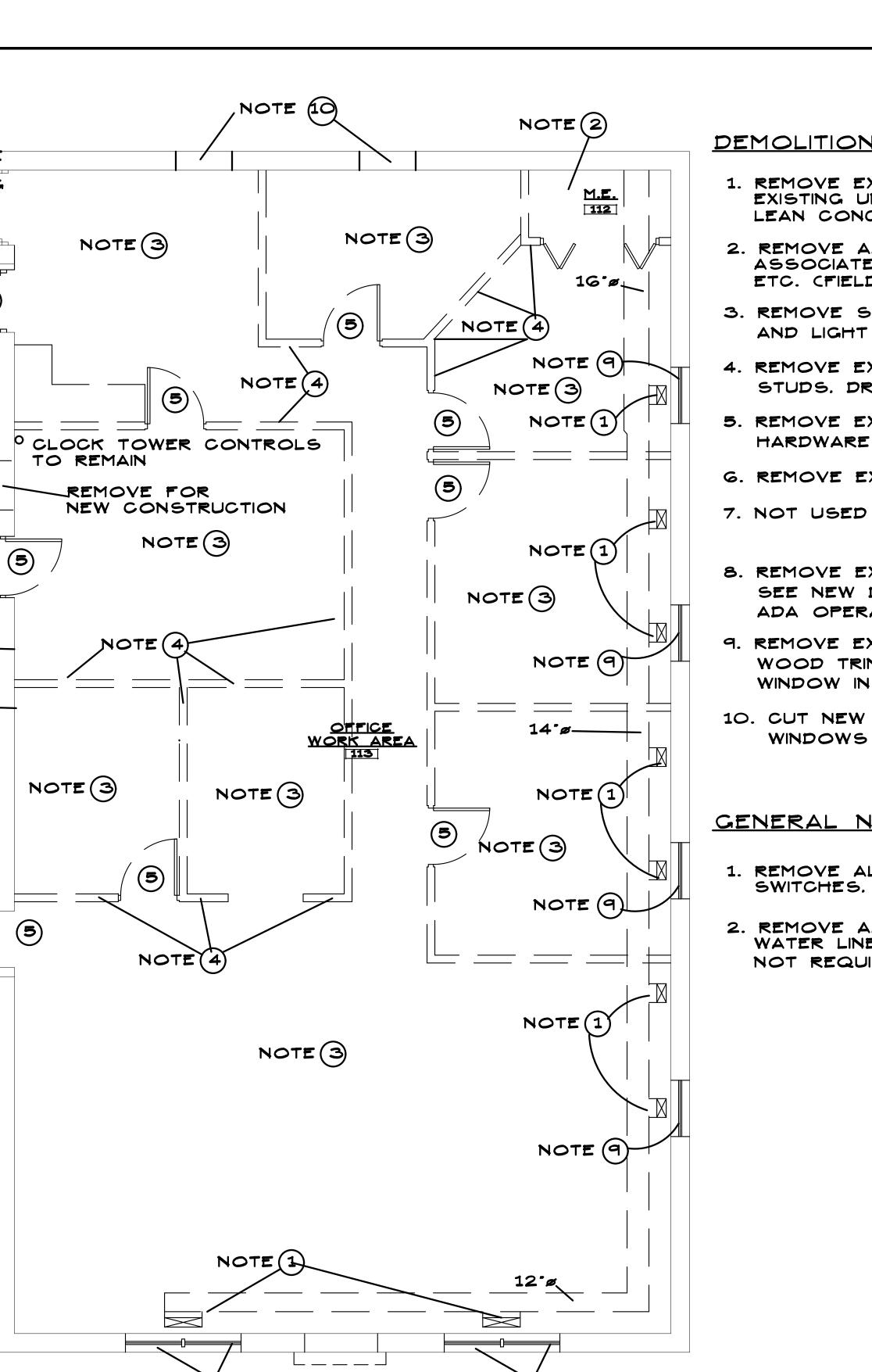
REMOVE CONCRETE SLAB AS SHOWN FOR NEW PLUMBING
